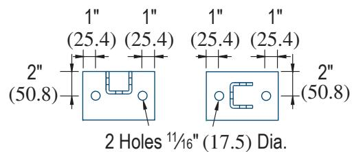
Standard Dimensions for 1 5/8" (41.3mm) width series channel fittings (Unless Otherwise Shown on Drawing)
