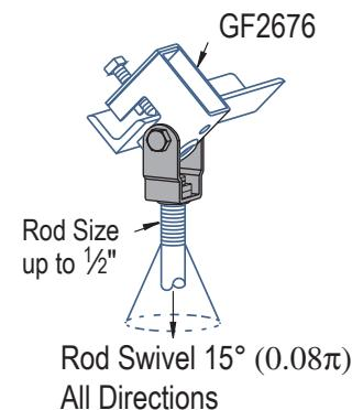
Clevis hanger to be used with GF2676 or GF2682 to provide angle adjustment and 15" (0.08π) free swing for up to 1/2" (12.7) rod suspension.
