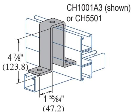
Standard Dimensions for 1 5/8" (41.3mm) width series channel fittings (Unless Otherwise Shown on Drawing)
