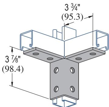
Standard Dimensions for 1 5/8" (41.3mm) width series channel fittings (Unless Otherwise Shown on Drawing)
