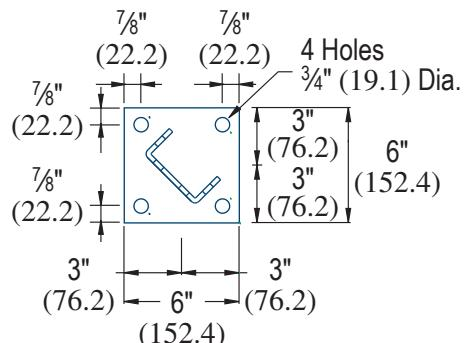
Standard Dimensions for 1 5/8" (41.3mm) width series channel fittings (Unless Otherwise Shown on Drawing)
