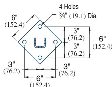
Standard Dimensions for 1 5/8" (41.3mm) width series channel fittings (Unless Otherwise Shown on Drawing)
