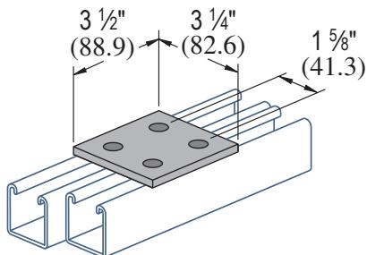
Standard Dimensions for 1 5/8" (41.3mm) width series channel fittings (Unless Otherwise Shown on Drawing)
