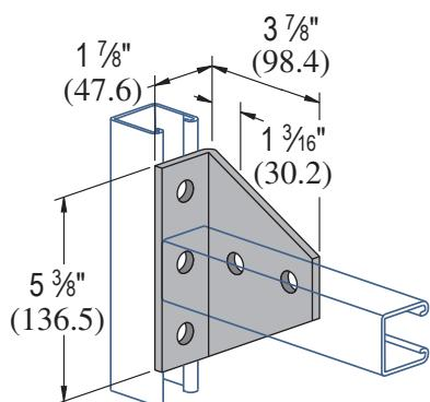
Standard Dimensions for 1 5/8" (41.3mm) width series channel fittings (Unless Otherwise Shown on Drawing)
