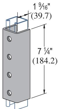
Standard Dimensions for 1 5/8" (41.3mm) width series channel fittings (Unless Otherwise Shown on Drawing)
