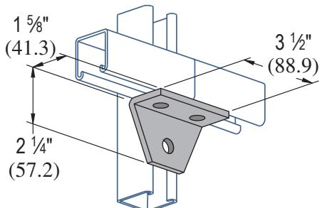
Standard Dimensions for 1 5/8" (41.3mm) width series channel fittings (Unless Otherwise Shown on Drawing)
