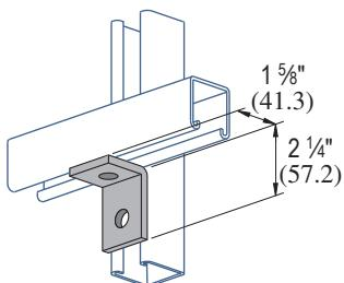
Standard Dimensions for 1 5/8" (41.3mm) width series channel fittings (Unless Otherwise Shown on Drawing)
