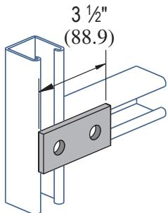
Standard Dimensions for 1 5/8" (41.3mm) width series channel fittings (Unless Otherwise Shown on Drawing)
