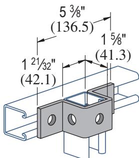
Standard Dimensions for 1 5/8" (41.3mm) width series channel fittings (Unless Otherwise Shown on Drawing)
