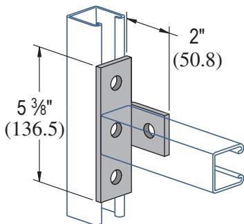
Standard Dimensions for 1 5/8" (41.3mm) width series channel fittings (Unless Otherwise Shown on Drawing)
