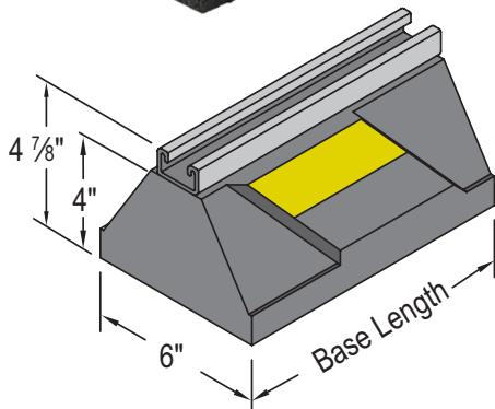
RTS Series channel support is designed for superior support of gas and refrigeration piping systems, cable tray, electrical conduit, multiple lines, HVAC equipment and many other applications.
