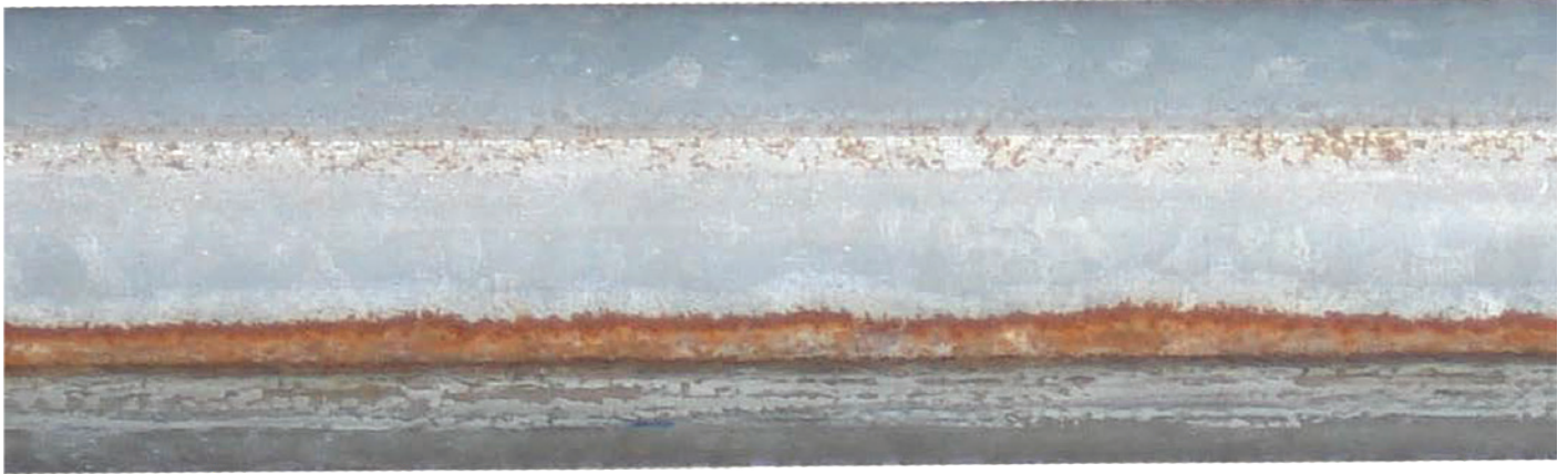
RED RUST ON RE-METALIZED WELD SEAM
